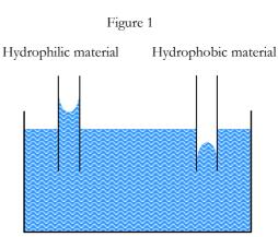
In the case of the <u>hydrophobic</u> materials, the meniscus is convex and the water level is <u>depressed</u> below that in the reservoir, as the water "tries to avoid contact" with the solid walls of the tube.
